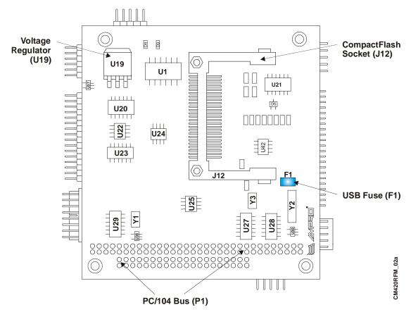
Figure 2-6. Connector Location (Bottom View)
